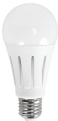
03A60-E27-18W Plastic housing+PC cover Wattage: 18W Lumen: 1700lm Voltage: AC220-240V 50/60Hz LED Type: 2835 SMD Beam angle: 230° Lamp base: E27 CCT: 2700-6500K PF: 0.5 Size: Dia60xH127mm Lifespan: 25000hrs
