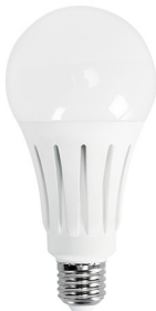
03A70-E27-20W Plastic housing+PC cover Wattage: 20W Lumen: 1800lm Voltage: AC220-240V 50/60Hz LED Type: 2835 SMD Beam angle: 230° Lamp base: E27 CCT: 2700-6500K PF: 0.5 Size: Dia70xH149mm Lifespan: 25000hrs
